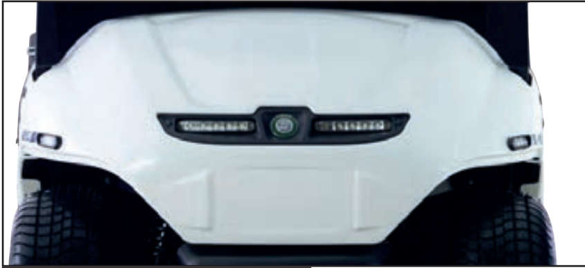
Standard LED Lighting System
