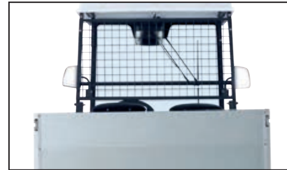
Driver Protection Steel Plate
